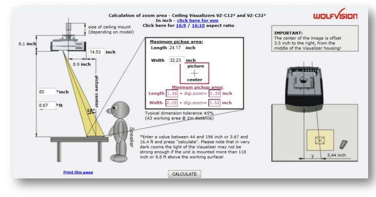
Determine mounting location of camera using the WolfVision online application in the Support Section of <u>www.wolfvision.com</u>.
