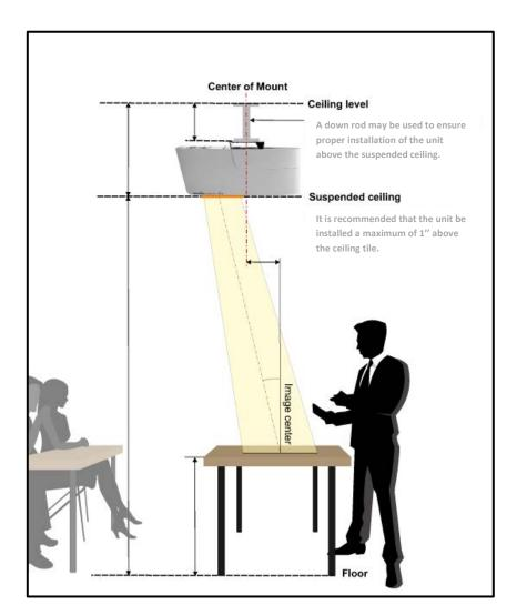
Determine mounting location of camera using the WolfVision online application in the Support Section of <u>www.wolfvision.com</u>.
