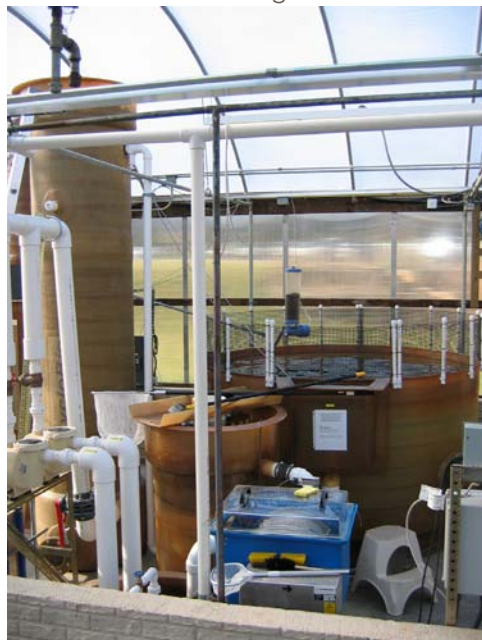
An individual RAS tank as part of the series of tanks used during this nitrate nitrogen study.
