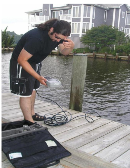
A volunteer uses the YSI 556 multiparameter instrument to measure several water quality parameters at once off the docks.
