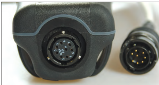
The YSI MS (military spec), waterproof, bayonet-style keyed connectors are far superior to plastic connectors.
