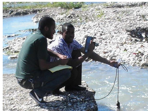
FAMV students using the YSI Pro Plus multiparameter water quality instrument in the Riviera Grise near SUH, FAMV campus. Students monitor basic parameters under the supervision of Dr. Nedunuri.
