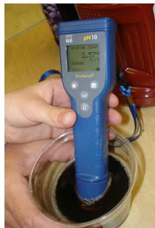
The pH10 for common household liquid pH values (above); The EcoSense pH100 with flat-tipped probe for soil (right)
