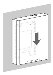
**NOTE**: To remove this unit from the mounting bracket, slide the unit in the opposite direction of installation while moving the UNLOCK switch on the rear panel (top edge in the illustration above) in the direction shown below.
