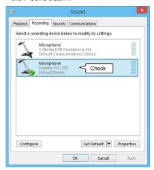
In most cases, simply connecting the product to a PC automatically sets "Yamaha YVC-330" as a default device.
