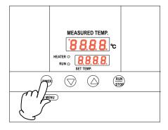
1 Press the TIMER key (SUBMENU key) long to enter the sub menu mode.
