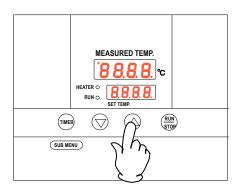
② "Off" is displayed on the set temperature screen. To lock settings, change to "on" using the ▲ key.
