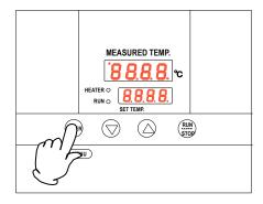
① Press the TIMER key (SUBMENU key) long to enter the sub menu mode.
