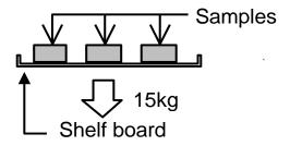
• Put instruments with appropriate spaces between them. Too many instruments may prevent proper temperature control. To assure proper temperature control, put instruments with a space at least 30% of the shelf board area.
