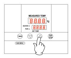
② "On" is displayed on the set temperature screen. The device keeps stop status after recovery from power outage when this setting is set to "off" using the ▼ key.
