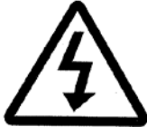
Warning high voltage
