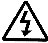
Danger!: High voltage
