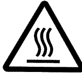
Danger!: High temperature
