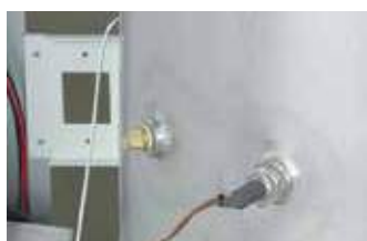
Standard equipped with 2 sensor ports on the main unit
