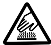
Caution: Burn Hazard!
