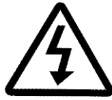
Danger!: High Voltage
