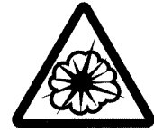
Danger!: Hazard of explosion
