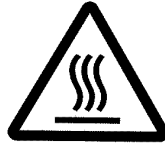
Danger!: High temperature
