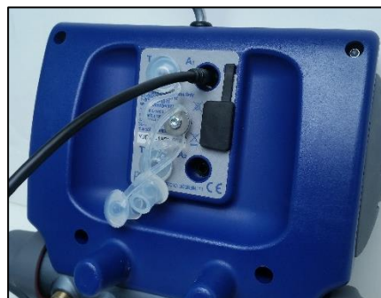
Figure 9: Connecting the Vacuum Sensor
