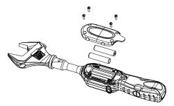
ATTENTION: When opening the battery cover of the wrench, you can see a viewing window for the water contact indicator. Through this viewing window, you can check if the wrench is damaged by water penetration where the water contact indicator turns red.
