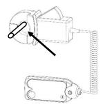
Depress the clamp lever and place the CT around the hot or neutral wire where AC current is to be measured. Make sure the clamp jaws are fully closed for best accuracy. If there is a ferrous metal surface near the placement of the clamp, the magnet on the bottom of the radio module can be attached to the surface for a more secure connection.
