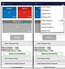
levels will be displayed. Pressures will be displayed as a large digital number to show measurement changes over time. If the system is initially at balanced pressure, the reading is displayed as 0 inWC (or other unit equivalent) until the system pressure differentials change from that level. From the Static pressure reading screen, a Filter Pressure Drop, Coil Pressure drop,
