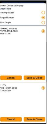
datasets that appear on the session readings screen, press the caret "^" icon next to each dataset to minimize or maximize it until the desired datasets are displayed. The system readings assignments are stored in the app memory for future sessions, but the assignments can be changed at any time by pressing on the reading that is to be changed.
