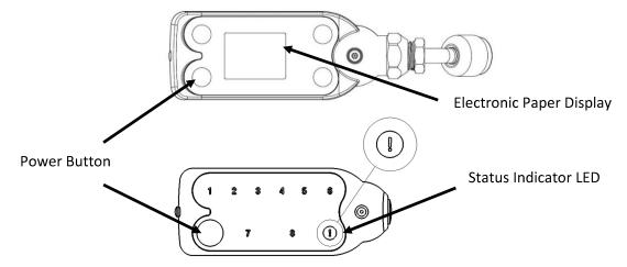
When using the YJACK PATH®, numeric LEDs 1-8 will illuminate to indicate the number of YJACK® and P51-870 TITAN® devices within range.
