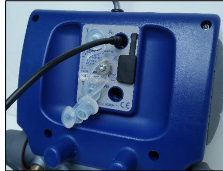
Figure 9: Connecting the Vacuum Sensor
