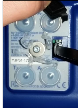
Figure 14: Connecting to the Micro-USB
