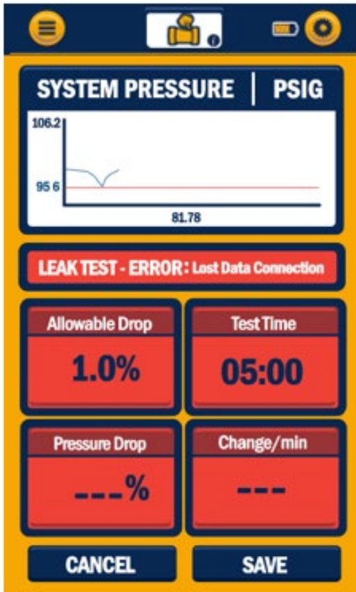
Figure 24: Pressure Decay Test - FAIL
