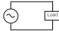
Single-phase 2-wire AC power supply and load are connected by two conducting wires
