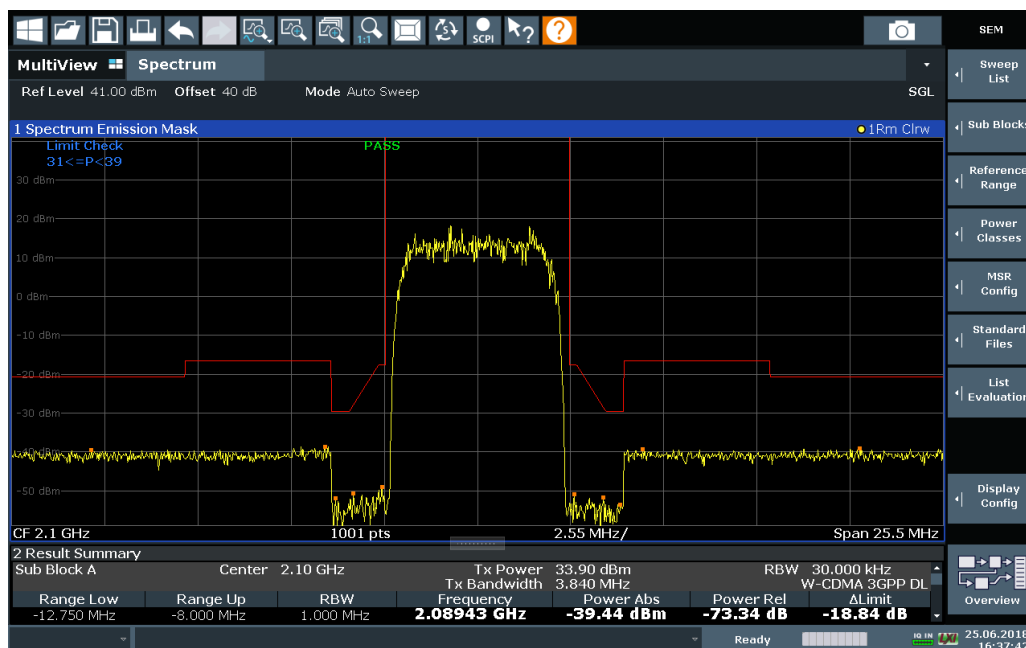
Figure 6-23: Detected peak display in SEM measurement
