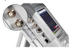
You can configure both BNC connectors for various applications. The name of the connector is printed on the insides of the protective caps.
