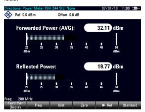
To get the best results, you should also define the frequency of the signal. For more information see "Measuring the Power with a Power Sensor" on page 69.
