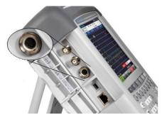
You can connect various accessories like the GPS receiver R&S HA-Z240 (order no. 1309.6700.02) to the AUX connector.
