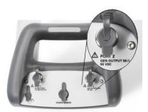
The tracking generator output power of the R&S ZVH is 0 dBm nominal.
