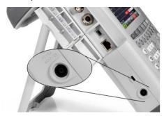
The R&S ZVH is supplied with power by the AC/DC transformer power supply via the DC connector. You can also use the DC connector to charge the battery.
