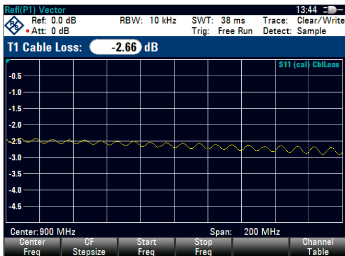
One-port cable loss measurement
