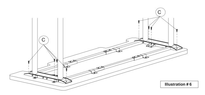
8.) Place a Lock Washer (J) on the two Locking Casters (A). Screw them into the front Leg mounting holes. Place a Lock Washer (J) on the two Non-Locking Casters (B) and screw them into the rear holes in the Legs. Tighten Casters using Caster Wrench (G).
