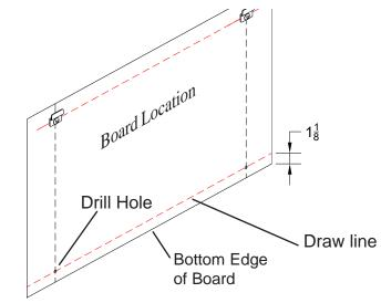
Lift and remove board from the Z-Hangers. Measure up from bottom line of board 1-1/8", and draw line as shown. Locate stud near each end of
