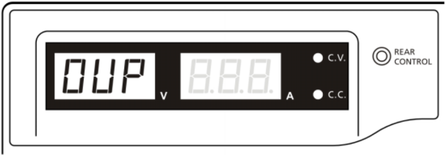
Figure 8 - Overt Voltage Protection
