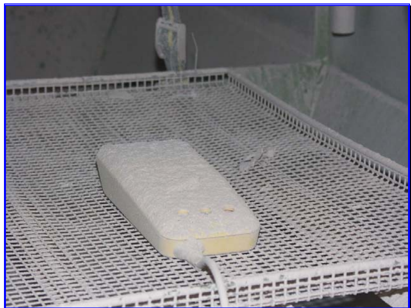
After the dust tightness test
