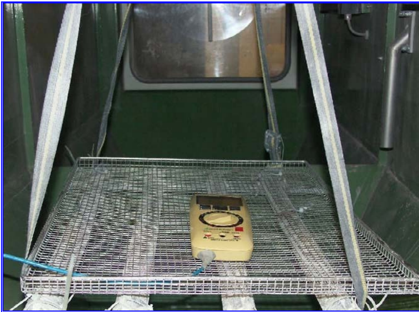
Emplacement – dust tightness test
