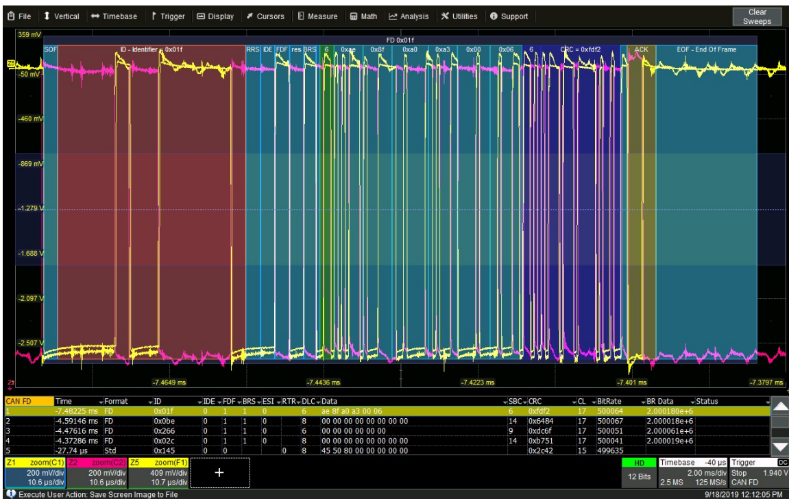
Figure 3: Touching a row in the Decode Results table opens a zoom of the corresponding packet with a color-coded overlay setting off and identifying the packet’s constituent parts.
