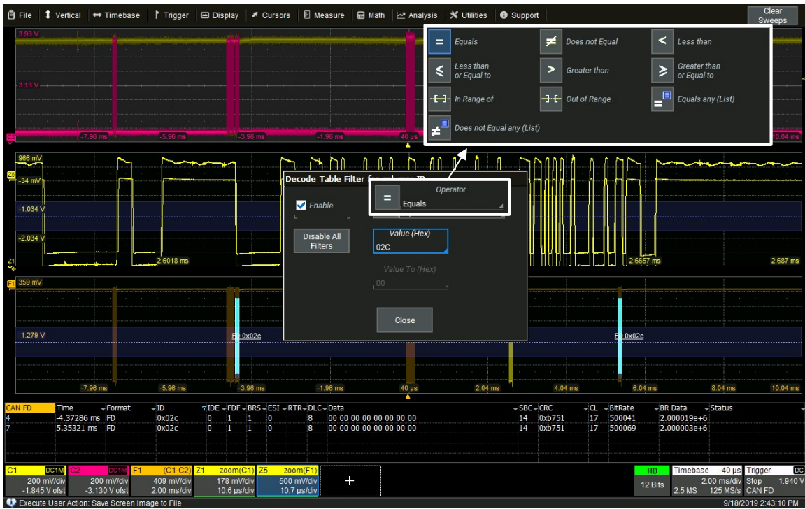
Figure 5: Applying conditional filters to the Decode Results table limits the display to only records meeting the filter criteria.
