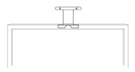
Attach the eBeam receiver to the bracket using the magnetic mounts on the bracket.
