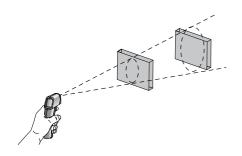
Ensure that the specific area or object to be measured is larger than the laser spot size of the device. The smaller the object the closer the equipment must be. For optimum measuring accuracy the area/object should be at least twice that of the spot size.
