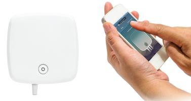
The EL-MOTE-T kit has been designed to monitor ambient temperature in a large range of applications, using a short probe at the base of the unit. Ideal for measuring ambient temperatures, the EL-MOTE-T is suitable for monitoring environments such as offices, warehousing and greenhouses.
