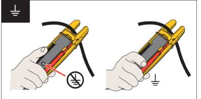
FieldSense technology works by providing a capacitive path from a contact point on the back of the tester and the operator's hand to earth ground.
