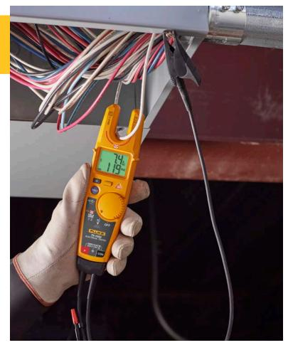
And since the measurement is performed through the cable's insulation, you reduce exposure to metallic conductors. You also decrease the potential for errors, or making contact with the wrong conductor.
