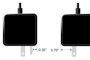
For power adapters with the grounding pin, measure from the edge of the adapter closest to the grounding pin. This dimensions must be 0.30" or less to fit on the 10 outlet power strip.
