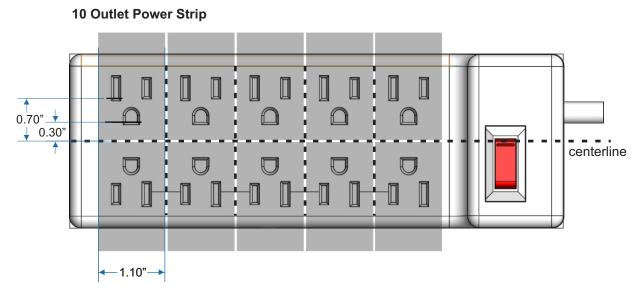
Adapter must be 1.1" wide or less to fit side by side on power strip.
