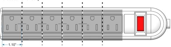
Adapter must be 1.1" wide or less to fit side by side on power strip.
