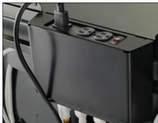
Power timer for charging (requires only 1 outlet to wall)
