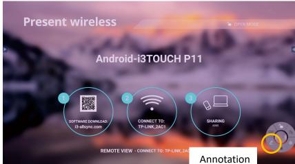
Please ensure the i3TOUCH is connected to the same network as your transmitting device, launch "Present Wireless" on the screen, scan the QR code or visit the download address to download and install i3ALLSYNC application on the transmitting device.
