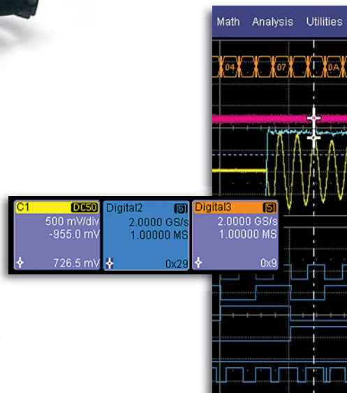
Use oscilloscope tools like horizontal and vertical cursors along with automatic measurements and statistics to measure analog and digital signals.
