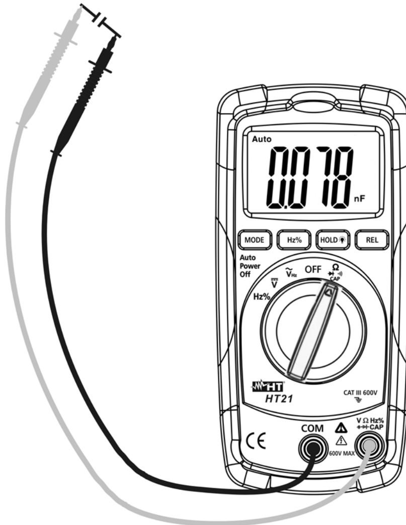
Fig. 7: Using the instrument for capacitance measurement
