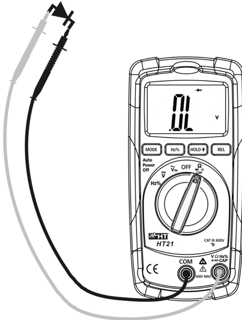
Fig. 5: Using the instrument for diode test
