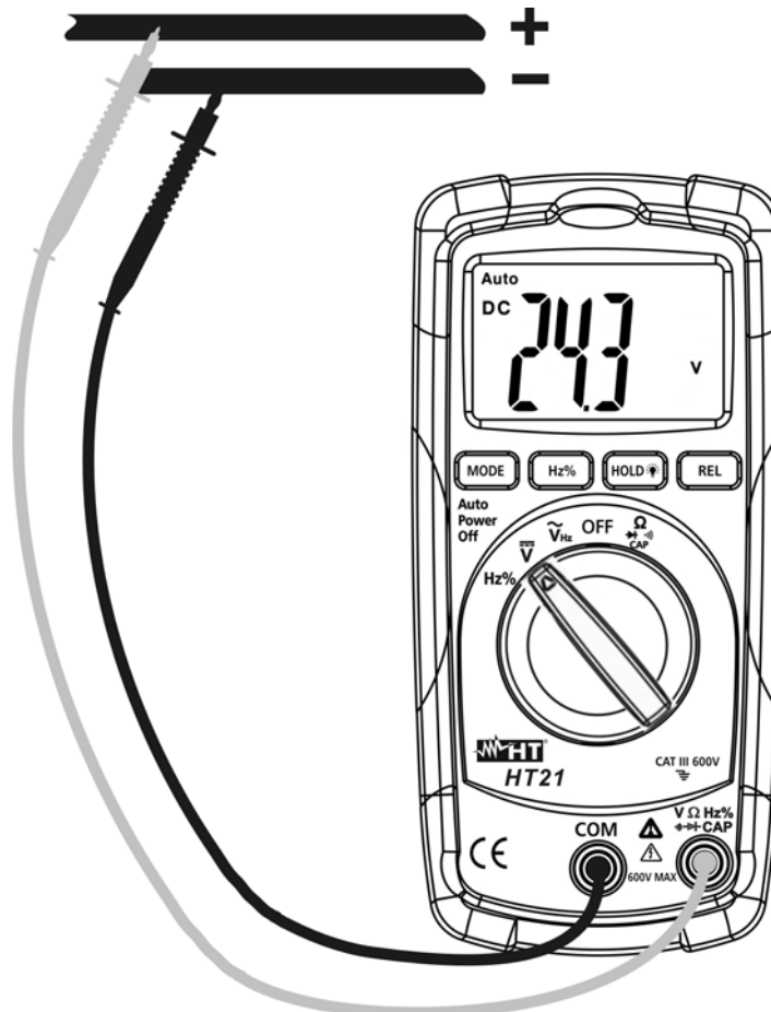
Fig. 2: Using the meter for DC voltage measurement
