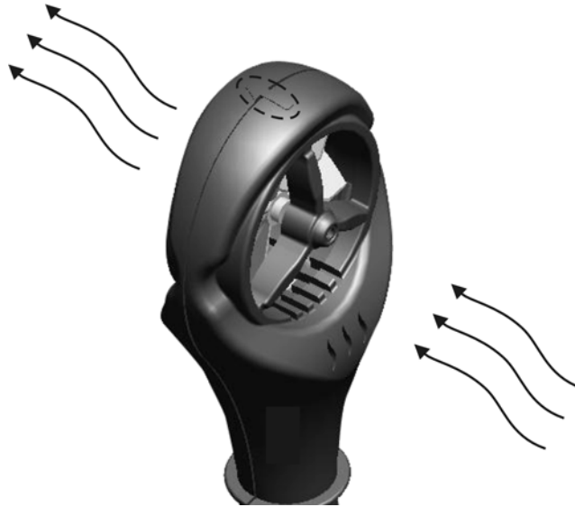
Fig. 3: Measurement of air speed and temperature/humidity
