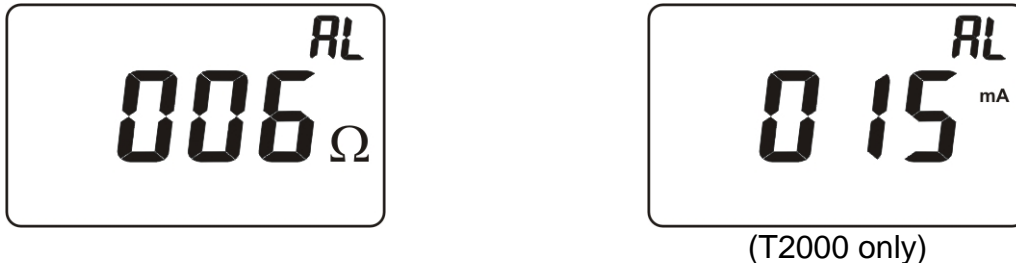
Fig. 39: Setting of alarm thresholds for resistance and current measurement
