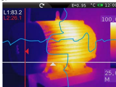
Fig. 26: Display of Measuring lines
