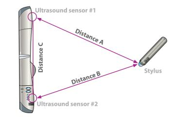
This process may become clearer through the analogy of thunder and lightning. If you count the number of seconds until you hear thunder after a lightning flash and then divide that number by 5, you can learn how many miles away a storm is. The process the mimio system uses to determine the stylus position on a whiteboard is similar.
