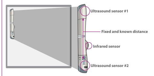
When a mimio Interactive Stylus touches the whiteboard, it triggers ultrasonic and infrared signals. The infrared signal travels instantly – at the speed of light – to the infrared receiver on the mimio bar. This signal lets the mimio system know that an ultrasonic signal was sent. When mimio Capture pens are used, the system can identify which pen touched the surface by an encoded signal.
