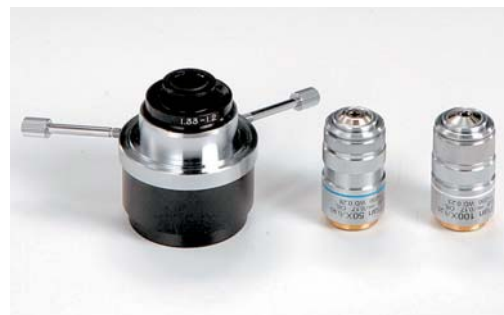
DARKFIELD CONDENSER AND OBJECTIVES WITH IRIS DIAPHRAGM
