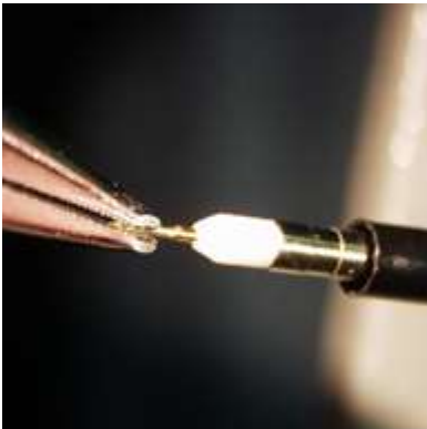
To remove tip, grip the spring-loaded portion of the tip beyond the outer sleeve and pull straight out.
