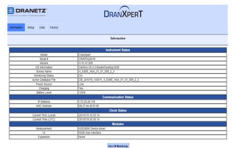
The Information page provides instrument status information, such as the serial number, firmware version, monitoring state, power source/battery charge status, IP address, and current time.
