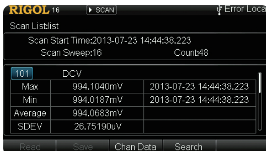
Display real-time scan information and all the measurement data of the channel selected
