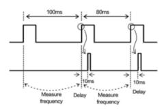
If the period of the external input is less than the setting of the delay time, the delay time is ignored and the ST-329 flashes as if the delayed time equals 0.
