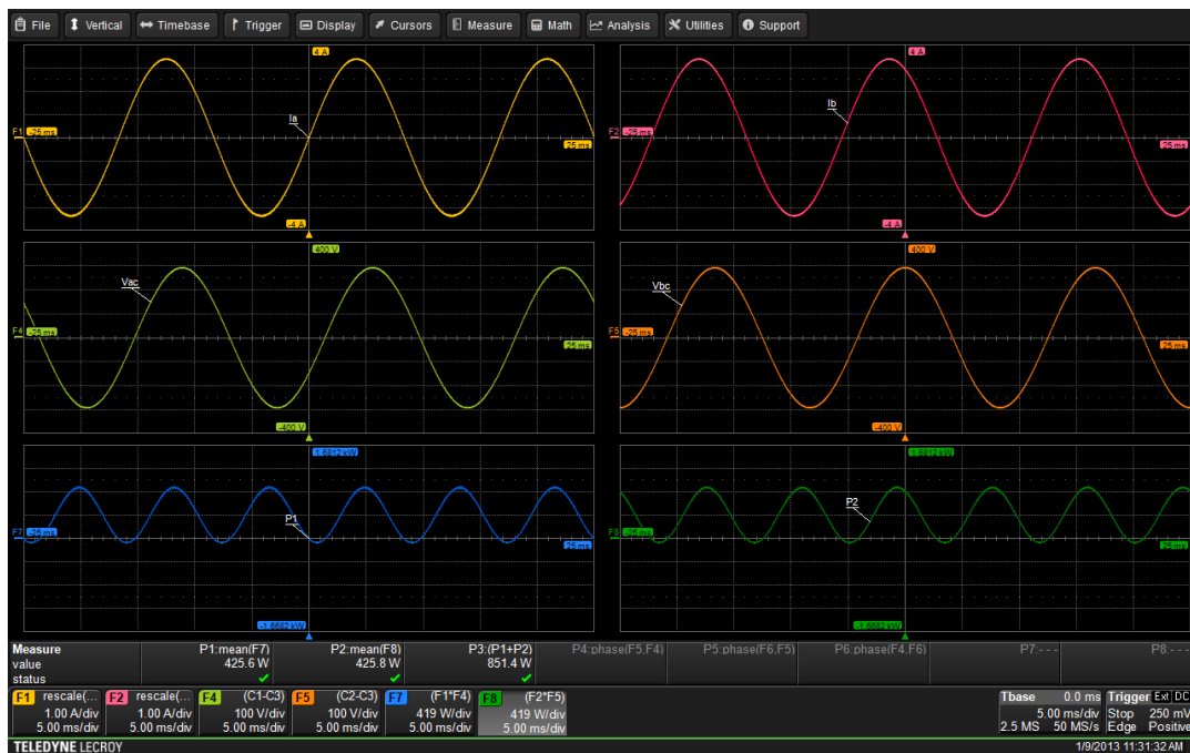
Figure 2: Computing the total power drawn by a three-phase motor using two line-to-line voltages and two phase currents
