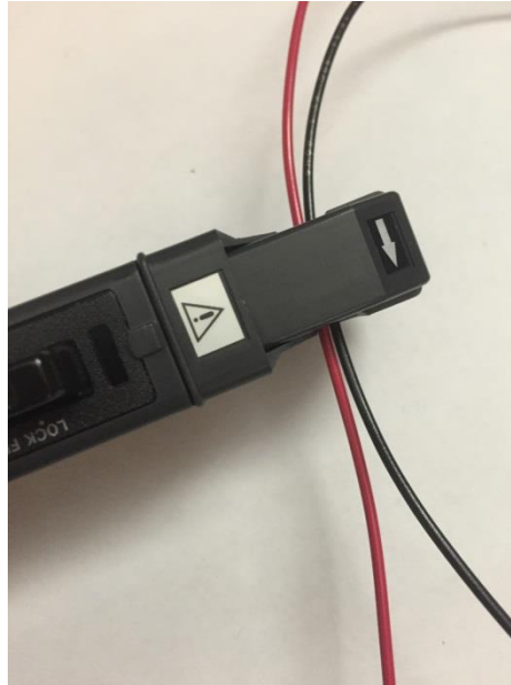
Figure 3: Setup for measuring the net current in a pair of conductors
